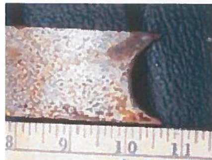
Fig 6. Curved end comes in 1/2 inch
