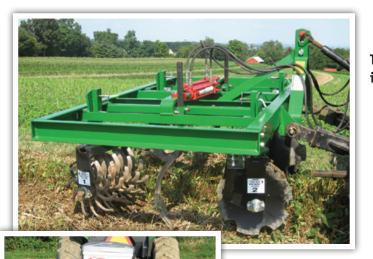
The primary cultivating tools mounted on the frame include rolling cultivators, disk gangs, coil tines, and optional fertilizer attachment.
