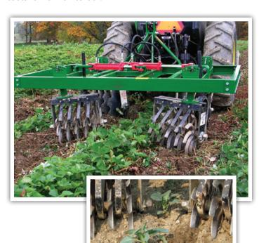
The hydraulic adjustment feature is particularly useful for cultivating close to the edges of plastic mulch.
