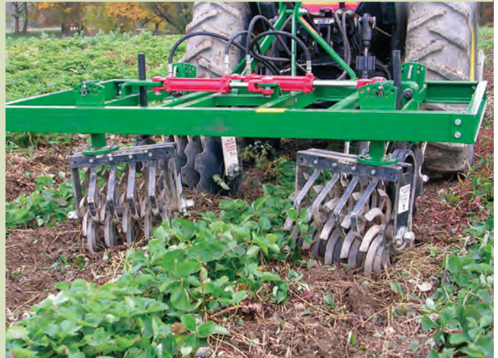
Rolling Cultivators are great for uprooting weeds and cutting through plant residue
