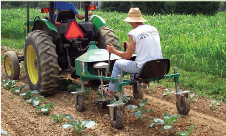
The PTO powered Eco Weeders are best for weeding between plants dramatically reducing hand work
