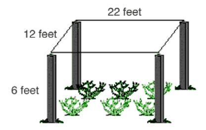
3.INSTALLATION - The netting can be draped over the plants, but we recommend installing a support structure. This will avoid entanglement of the net in the branch tips.
