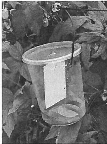
Monitoring trap for SWD. A plastic container with holes, containing apple cider vinegar as a bait, and a sticky trap to catch flies. Traps may also be used without the yellow sticky trap if a drop of unscented soap is added to the apple cider vinegar. With this method, count the flies in the liquid and replace the liquid each week. Photo: Rufus Isaacs.
