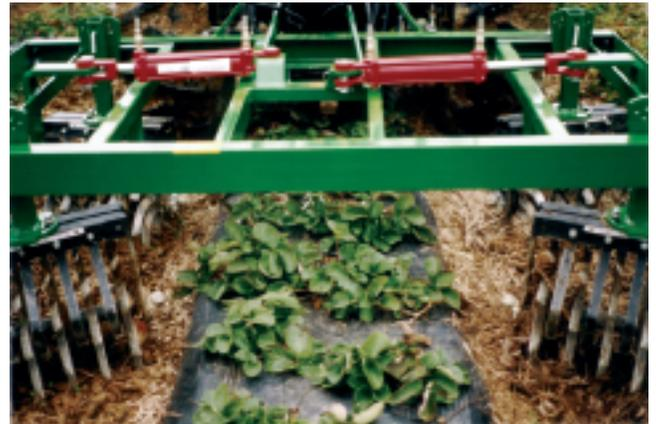
The cultivator frame consists of two channels which form the track for two sliding sub frames. The cultivating tools are mounted on the sub-frames and are hydraulically adjusted by the tractor operator. With this adjustment fine tuning of the cultivator to size of the crop size is done quickly when moving between different fields. This feature is especially useful for cultivating the edges of plastic mulch. The rolling cultivators move the soil laterally
